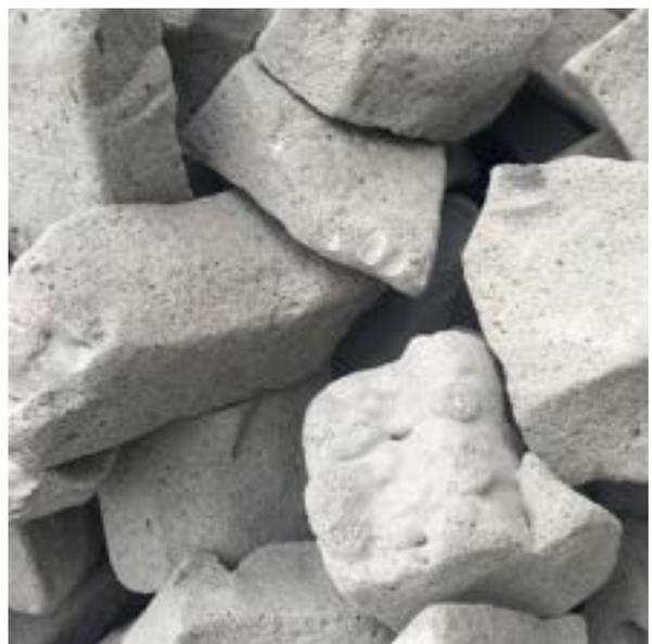
**Figure 2.** Ultra-Lightweight Foamed Glass Aggregate (UL-FGA) is made from 100 percent post-consumer recycled glass.
