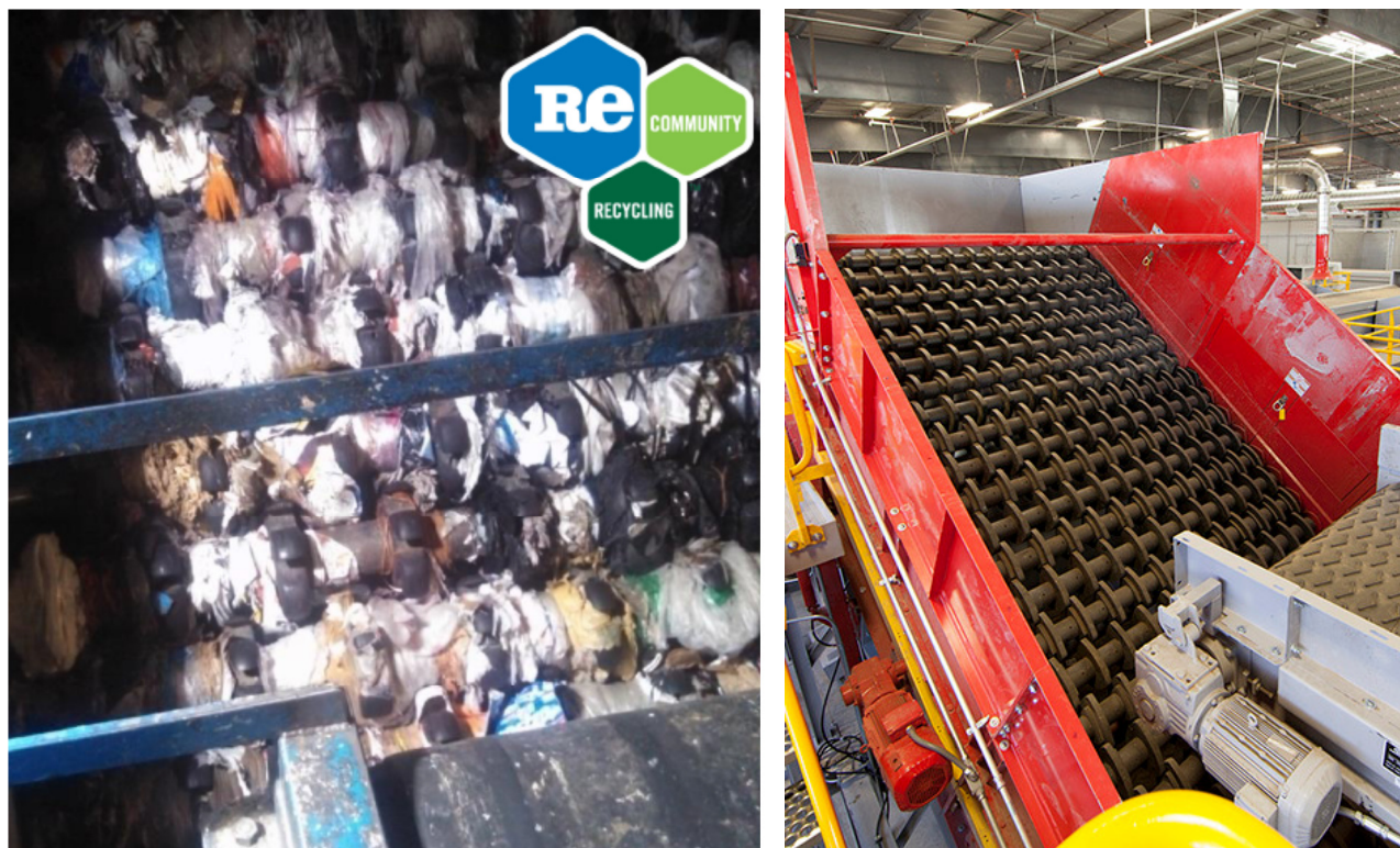
Figure 10 – A Film-Fouled Screen and a Clean Screen
