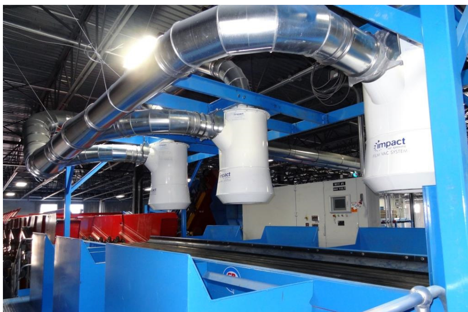
Figure 18 – Film Vacuum Takeaway System for Manual Film Sorting
